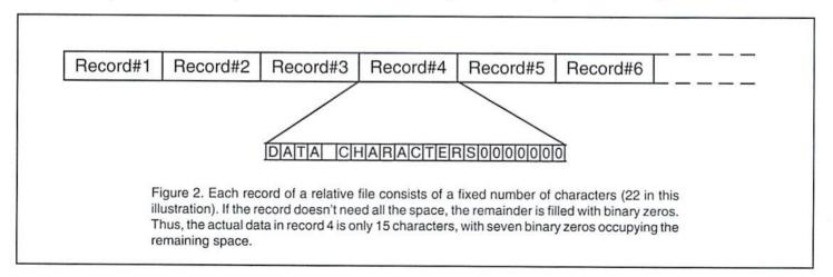
If a program has just written a record and now wants to move to a different one, a lot of work must take place within the drive. First, the record we have just "written" has not yet been put on the disk; it's still in RAM buffers. So the drive needs to write up to three blocks before it can shift its pointers and look for the different record.
